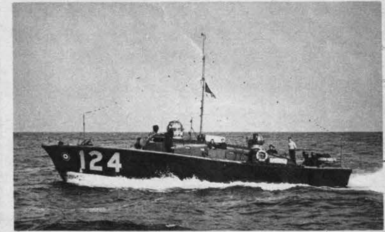
U.S. Lend-Lease supplies Britain with this 63-ft. high-speed launch. It has a long, low streamlined cabin and two machine-gun turrets. Undulant deckline is high, sheer forward, drops to pointed clipper bow.
